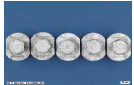
Fig. 19: Connector part with multilayer coating (organic flake topcoat) after ten weeks in the ISO 20340 test with UV radiation.
