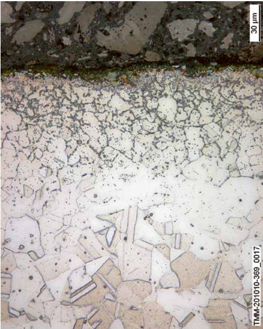
Fig. 11: Scanning electron micrograph image of a selective attack Welded zone of a 1.4401, (A4, 316) material.
