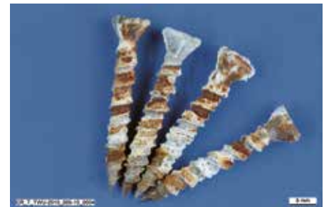
Fig. 14: Electrogalvanized screws with around 5 µm zinc coating after 48 h (up) and 96 h (down) in the salt spray test.
