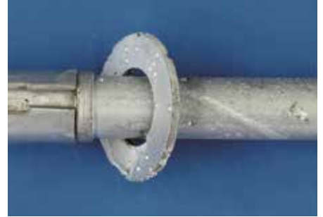
Fig. 5: Example of pitting corrosion on a stainless steel product.
