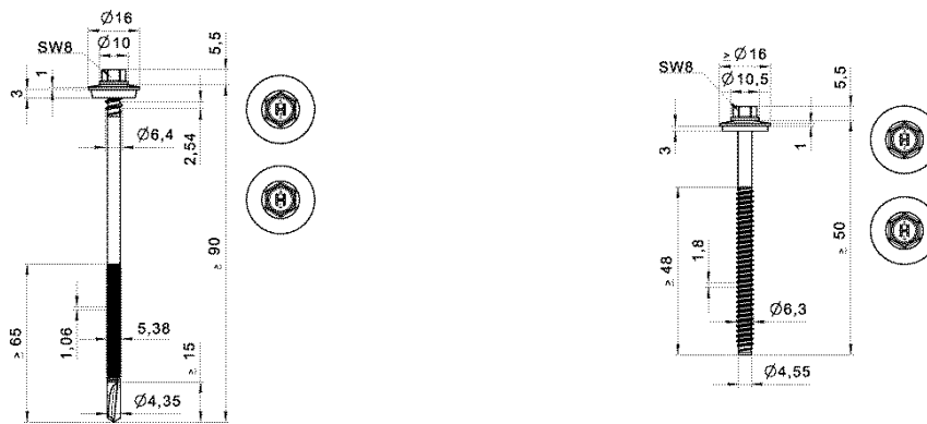
Figure 1: Fastening screws for sandwich panels (exemplary)
