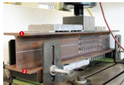
1 Compression flange 2 Tension flange
