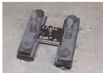
X-BT on 8.0 mm base plate
