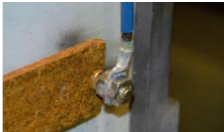
Test assembly X-BT with double nut
