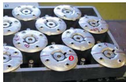
3 Markings to measure disc rotation
