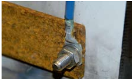
Test assembly X-BT with cable lug
