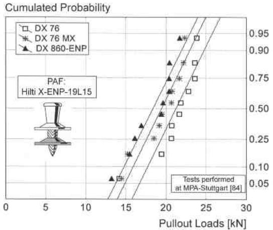
**Figure 95.** Pullout resistance on 20 mm thick base steel
