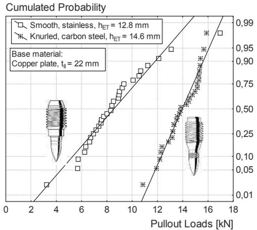
**Figure 39.** Loading capacity of threaded studs set in a copper plate
