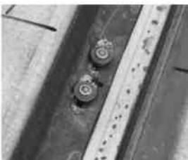
Figure 61. Hole elongation during cyclic shear loading tests
