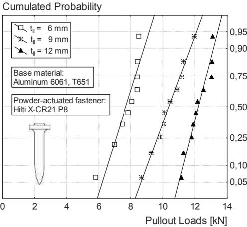
**Figure 38.** Example of the loading capacity of stainless steel powder-actuated fasteners in aluminum
