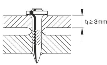
**Figure 70.** Formation of a gap between component I with  $t_1 \geq 3$  mm and component II
