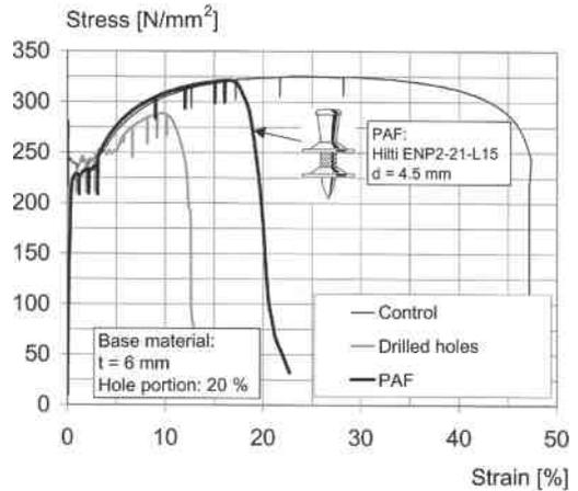
Figure 41. Stress-strain characteristics of steel with low tensile strength
