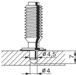
Figure 8. Blunt tip powder-actuated fastener Hilti X-BT after driving
