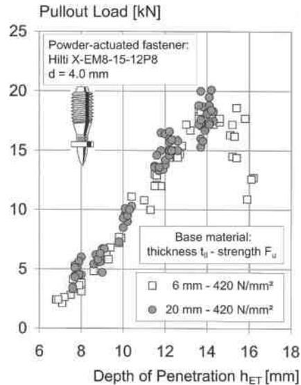
Figure 18. Influence of depth of penetration in base materials with a thickness of 6 mm or 20 mm
