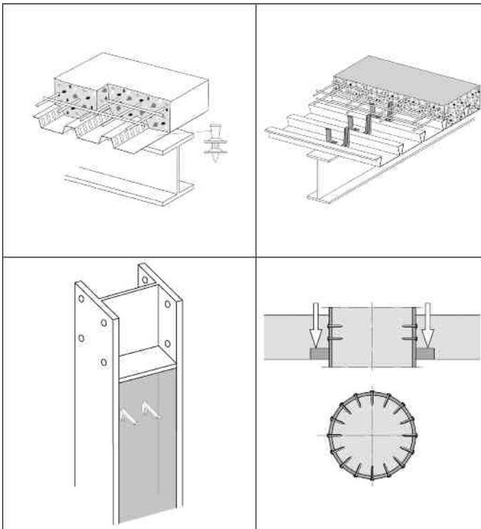
**Figure 84.** Use of powder-actuated fasteners in composite structures
