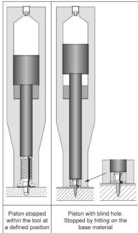
Figure 20. Piston brake concepts
