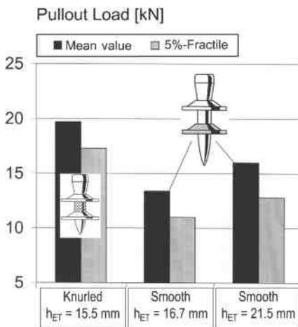
Figure 26. The influence of knurling on the fastener
