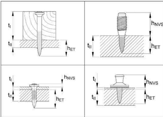
**Figure 9.** Components I and II, depth of penetration  $h_{ET}$  and fastener stand-off  $h_{NVS}$ . Component I: fastened component, thickness  $t_I$ . Component II: base material, thickness  $t_{II}$ .
