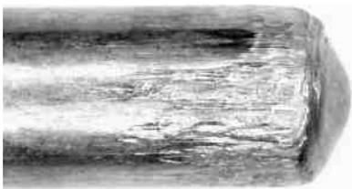
Figure 14. Base material adhering to a pulled-out fastener
