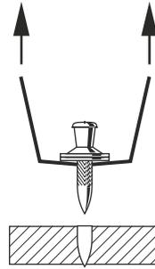
Figure 11. Anchorage failure
