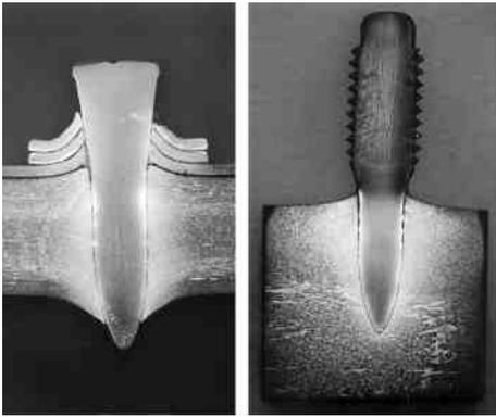
Figure 2. Ground cross-sections of fasteners after driving
