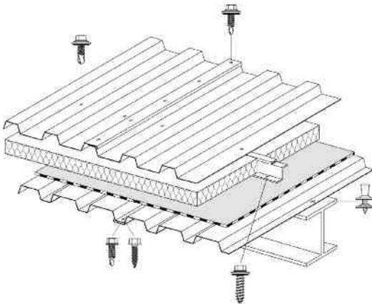
Figure 46. Typical composition of a lightweight metal structure
