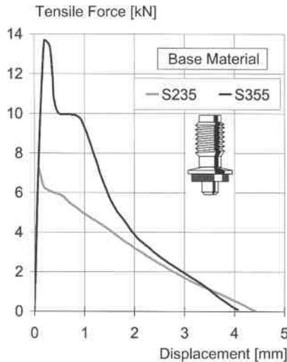
Figure 16. Load-displacement curves for blunt tip fasteners Hilti X-BT in solid steel
