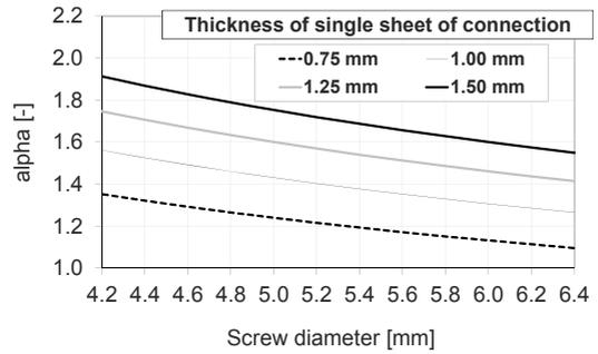
Figure 90. Coefficient  $\alpha$  for screw-fastened joints in accordance with Table 8.2 from EN 1993-1-3 [64] with  $t_I = t_{II}$
