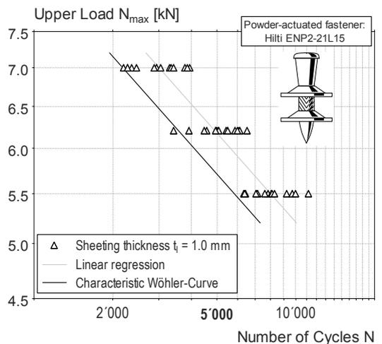
**Figure 93.** Example of the dynamic pullover resistance of a connection made with a powder-actuated fastener with a sheet metal thickness  $t_1$  of 1.0 mm
