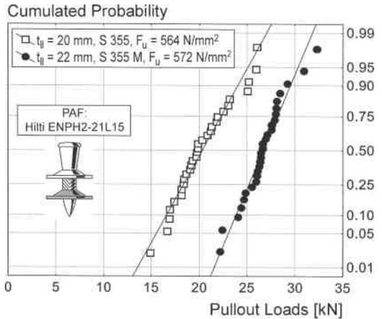
**Figure 107.** Loading capacity of the anchorage in thermomechanically-rolled steel ( $t_t = 0.75$  mm)
