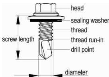
**Figure 47.** Fastening screw designations
