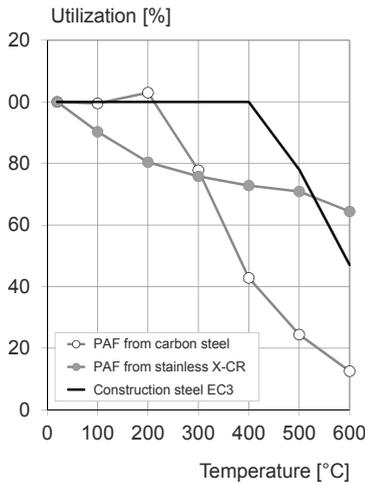
Note: The line representing construction steel shows the influence of temperature on the yield point in accordance with [27].
