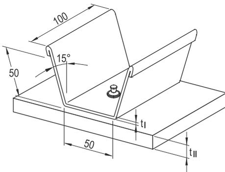
**Figure 91.** Shape of sheet specimen for tensile testing of sheeting
