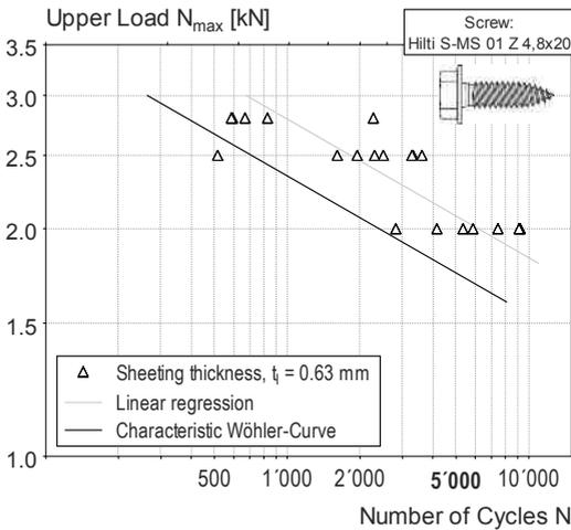
**Figure 94.** Example of the dynamic pullover resistance of a screw fastening with a sheet metal thickness  $t_s$  of 0.63 mm
