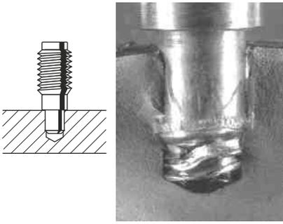
Remark: The photograph shows the fractured area of the base material after a fatigue test.
