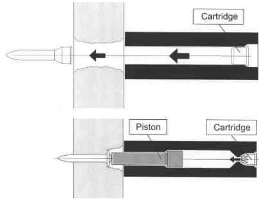
Figure 4. High-velocity tool principle versus low-velocity piston principle
