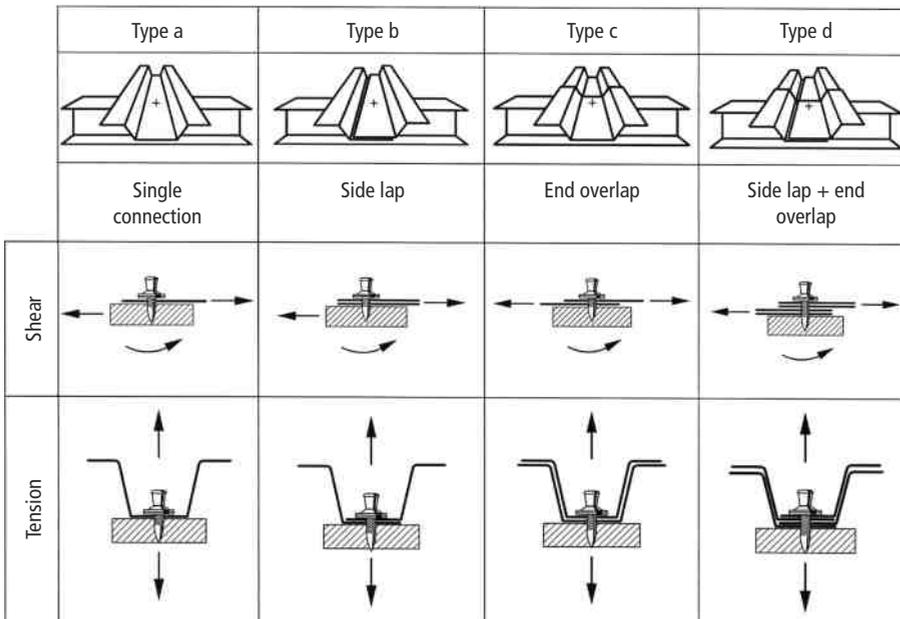
Figure 63. Types of fastening and loading
