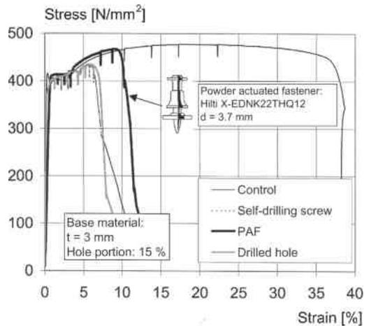
Figure 40. Stress-strain characteristics of steel with high tensile strength
