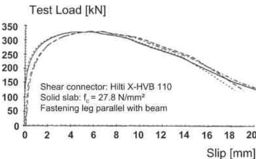
Figure 86. Load-displacement diagrams for the X-HVB shear connector [117]
