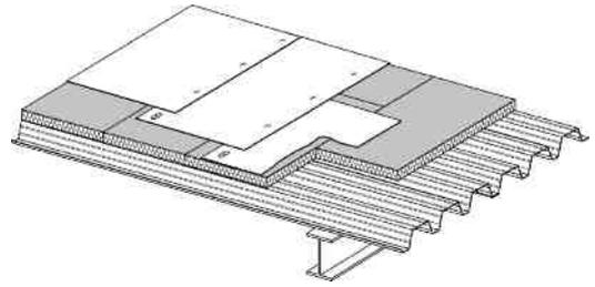
**Figure 81.** Roof composition with sealing membrane and integrated thermal insulation
