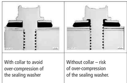
Figure 55. Screws with sealing washer, with and without collar
