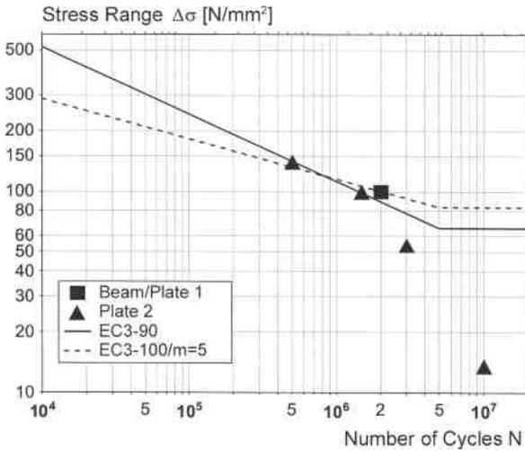
Figure 35. Stress ranges corresponding to the loading protocol
