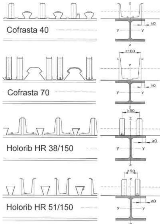
Figure 87. Optimum positioning of X-HVB shear connectors
