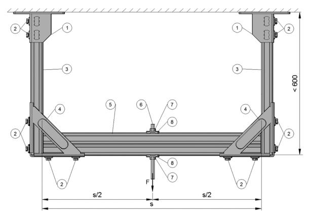
Trapeze frame with s = 700 mm, 1000 mm, 1250 mm and centric connection for load introduction
