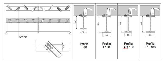
Minimum section width = 40 mm (e.g. old section IAO 100), Minimum centre distance of steel sections = 400 mm
