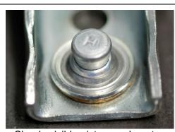
Clearly visible piston mark on top washer
