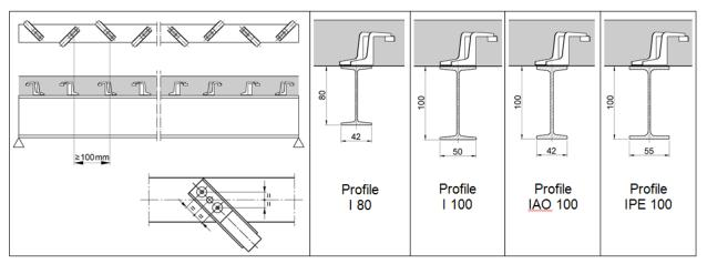
Minimum section width = 40 mm (e.g. old section IAO 100), Minimum centre distance of steel sections = 400 mm
