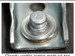
Clearly visible piston mark on top washer
